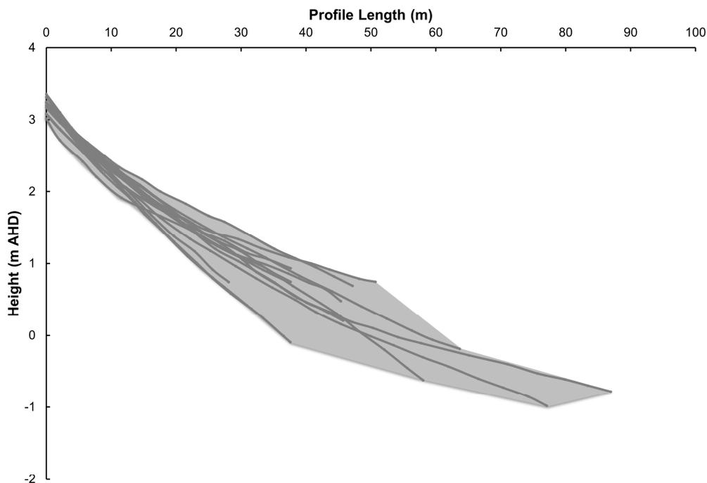
**Figure 5. Profile envelope in grey for the GPR beachfaces shown in Figure 3.**
